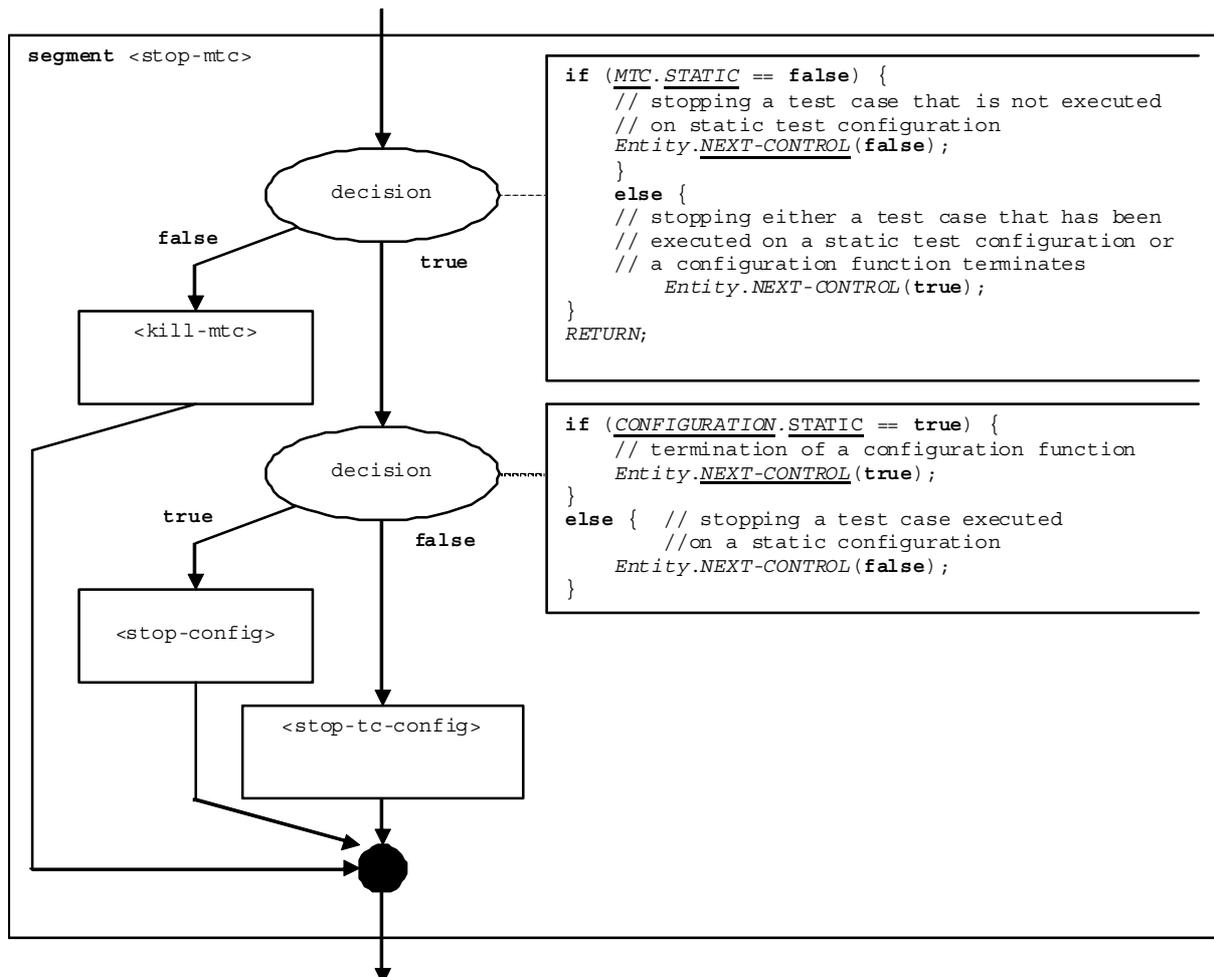
Figure 125a of ES 201 873-4 [2]: Flow graph segment <stop-mtc>
