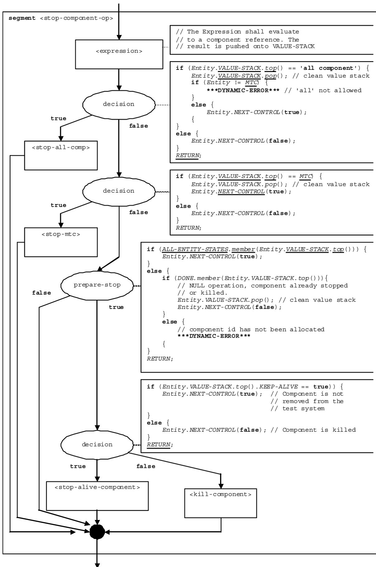
Figure 125 of ES 201 873-4 [2]: Flow graph segment &lt;stop-component-op&gt;
