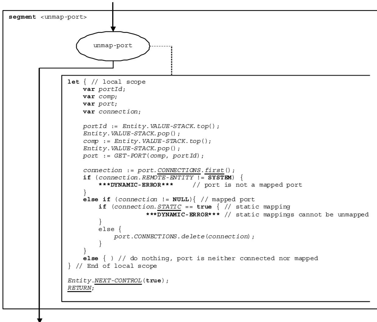
Figure 136c of ES 201 873-4 [2]: Flow graph segment <unmap-port>
