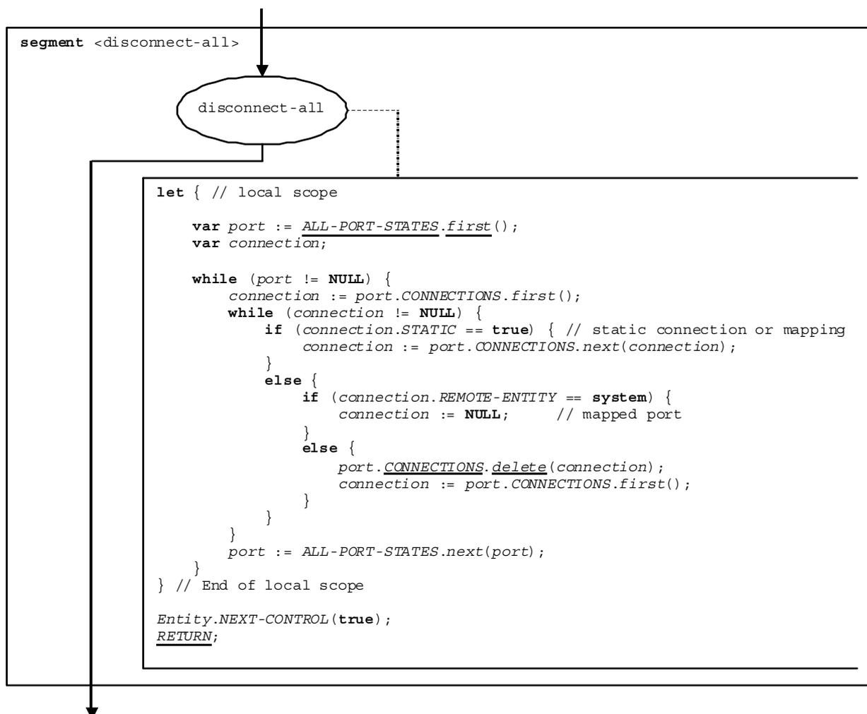
Figure 64b of ES 201 873-4 [2]: Flow graph segment <disconnect-all>
