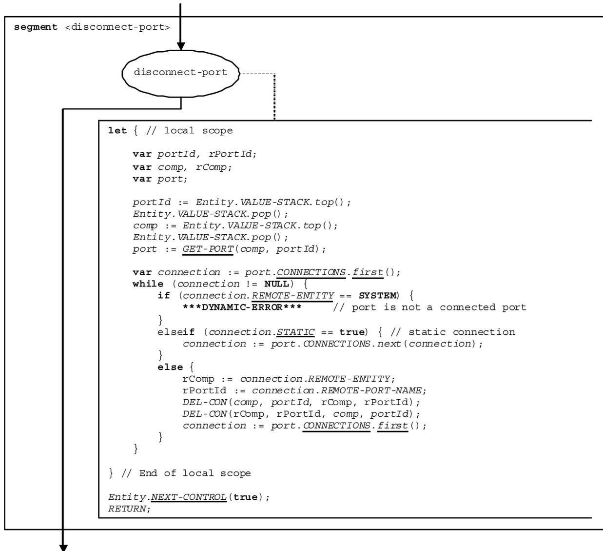
Figure 64d of ES 201 873-4 [2]: Flow graph segment <disconnect-port>
