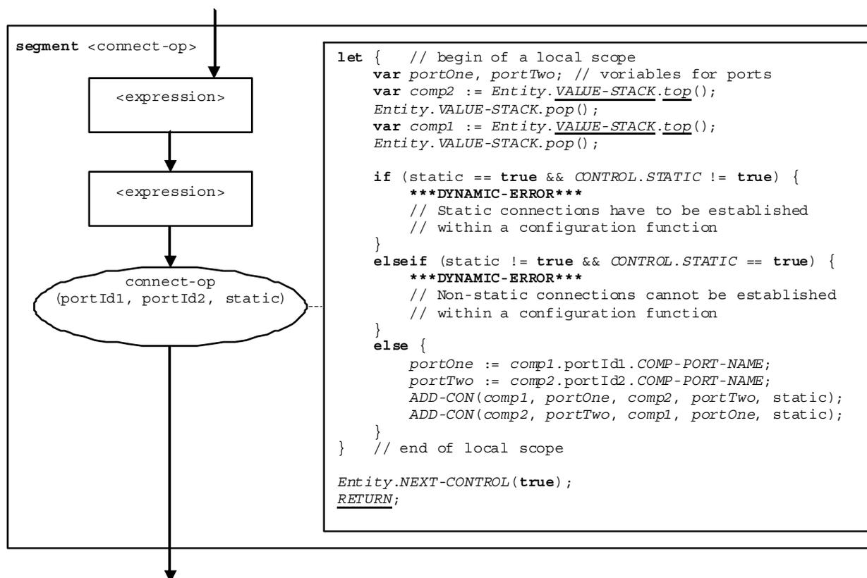
Figure 60 of ES 201 873-4 [2]: Flow graph segment `<connect-op>`
