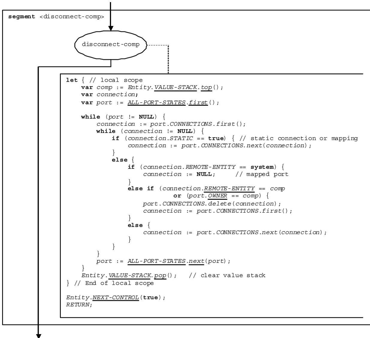
Figure 64c of ES 201 873-4 [2]: Flow graph segment <disconnect-comp>
