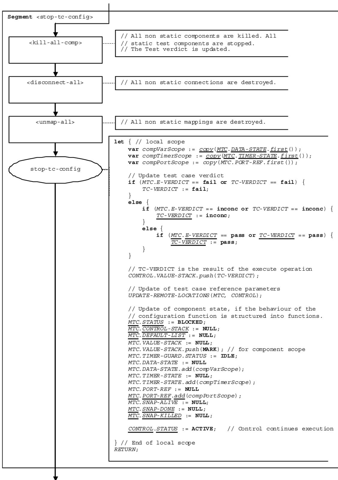
Figure 127b of ES 201 873-4 [2]: Flow graph segment &lt;stop-tc-config&gt;
