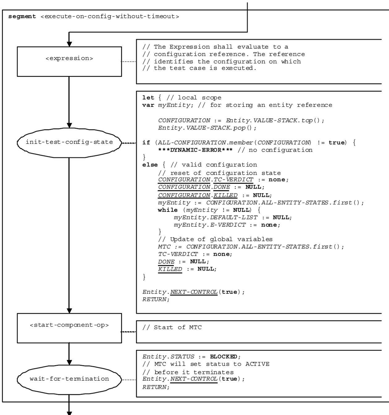
Figure 69b of ES 201 873-4 [2]: Flow graph segment <execute-on-config-without-timeout>
