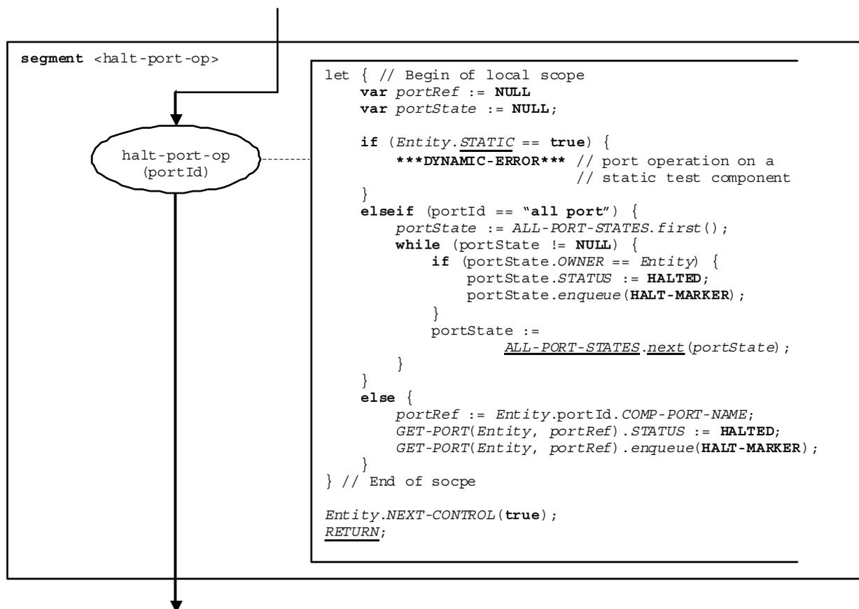
Figure 89a of ES 201 873-4 [2]: Flow graph segment <halt-port-op>
