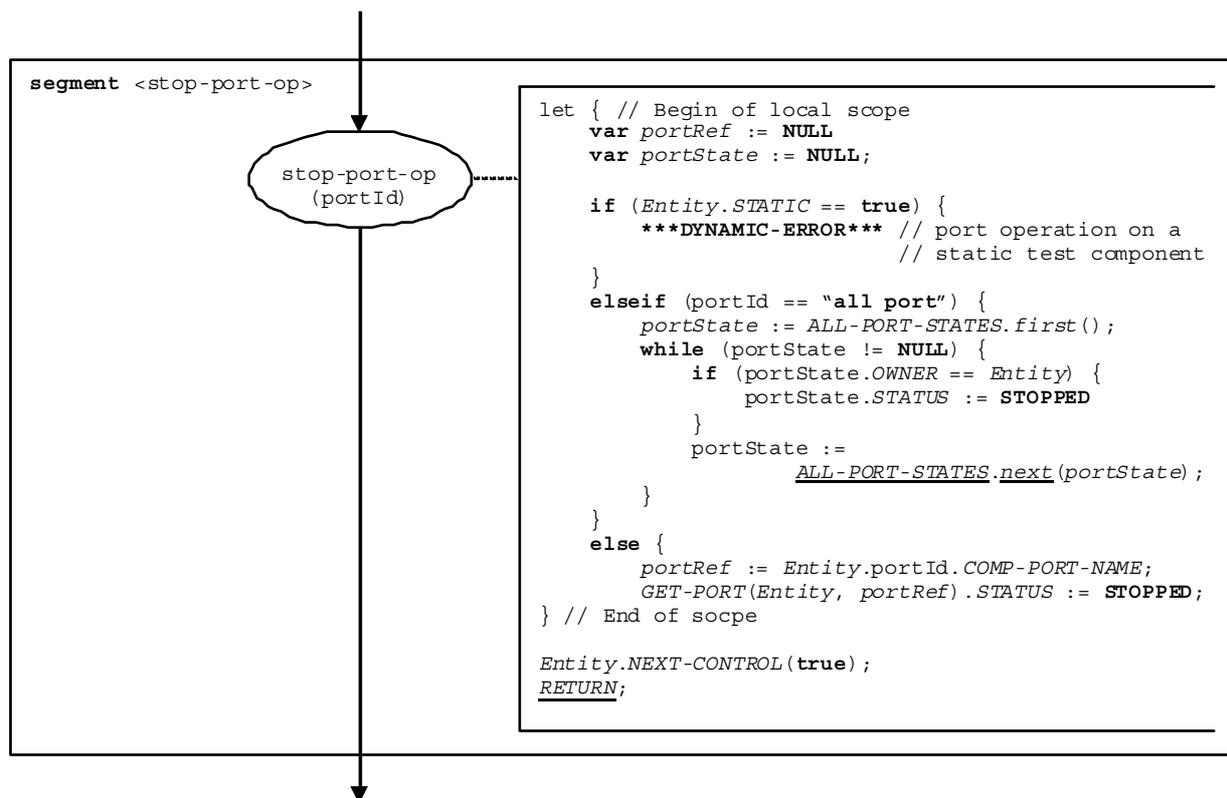
Figure 129 of ES 201 873-4 [2]: Flow graph segment <stop-port-op>
