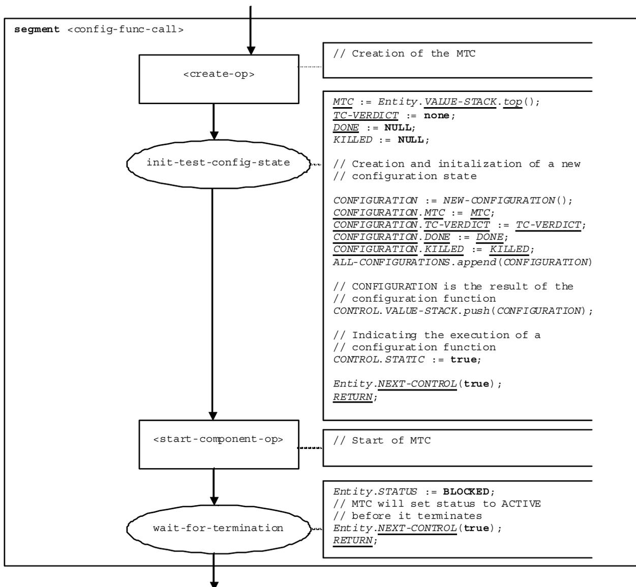
Figure 59a of ES 201 873-4 [2]: Flow graph segment <config-func-call>
