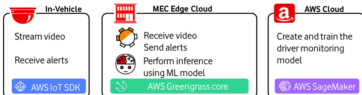
The in-vehicle Raspberry Pi video stream application has been built using the AWS IoT SDK, which establishes a secure communication between the device and the AWS Greengrass instance at the edge. Video streams are sent in MQTT messages between the Raspberry Pi and AWS Greengrass over the wireless network.
