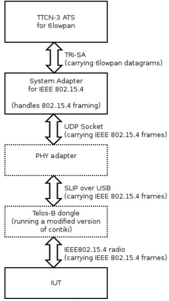
*Figure 2: Example of physical adapter implementation using a Telos-B dongle*
