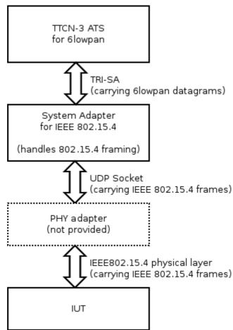
Figure 1: Framework of the System Adapter
