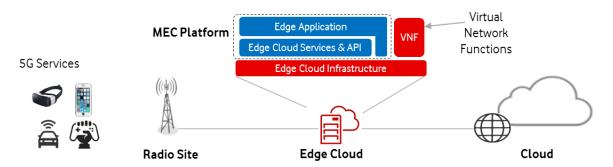
In above use case, an automotive application has been deployed in a three-tiered way using i) a simple device platform (Raspberry Pi), ii) a cloud computing environment at the network edge that is also available in a public cloud (AWS's Lambda function environment) and iii) the public cloud itself (which supports the same Lambda function environment).
